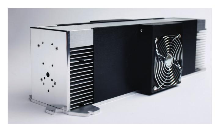
**Iradion** is dedicated to the development and manufacture of custom Colasers for applications in Industry, Medicine, and Science. Iradion Laser's employ a ceramic based, "inside out" concept placing all the reactive metal components outside the ceramic vacuum enclosure. This approach makes it far easier to build, much more reliable, and longer lasting.
